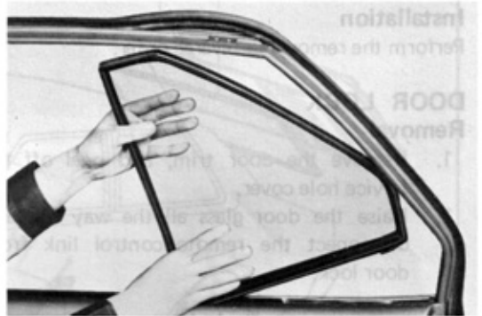
Fig. 2-57 Removing Quarter Window Glass
