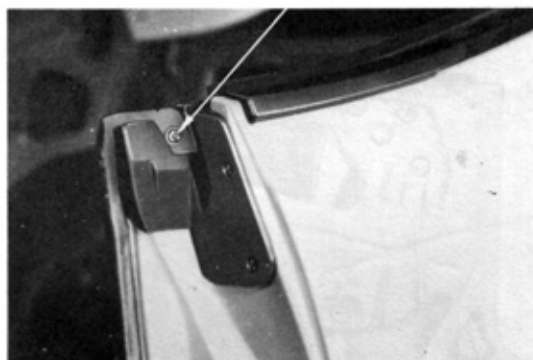
Fig. 2-124 Door Trim Board Removal (2)
