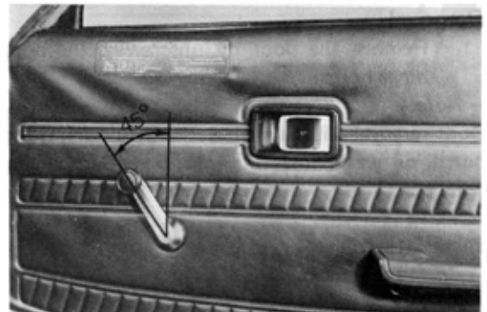
Fig. 2-34 Regulator Handle Installed Angle
