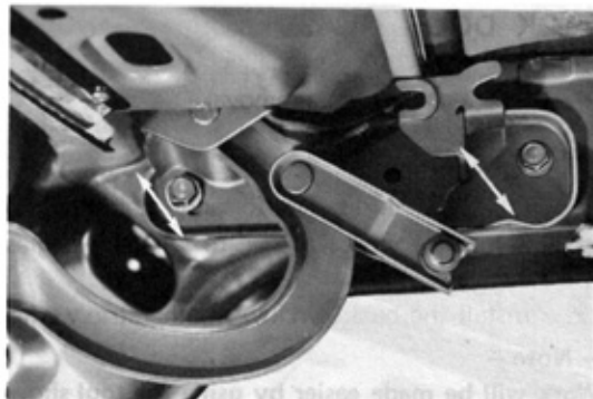
Fig. 2-156 Back Door Adjustment
