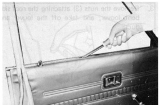
Fig. 2-92 Removing Door Belt Moulding
