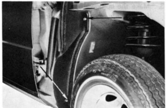
Fig. 2-8 Removing Splash Shield
