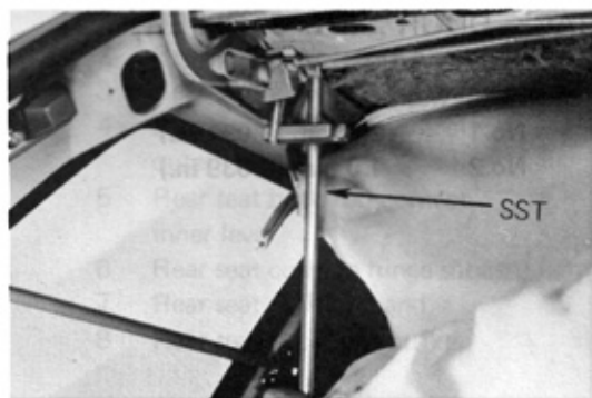
Fig. 2-154 Removing Torsion Bar
