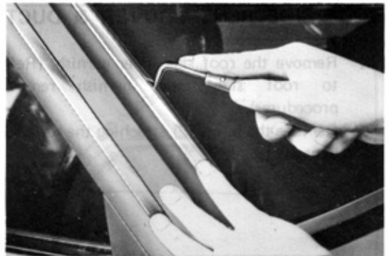
Fig. 2-91 Installing Windshield Moulding
