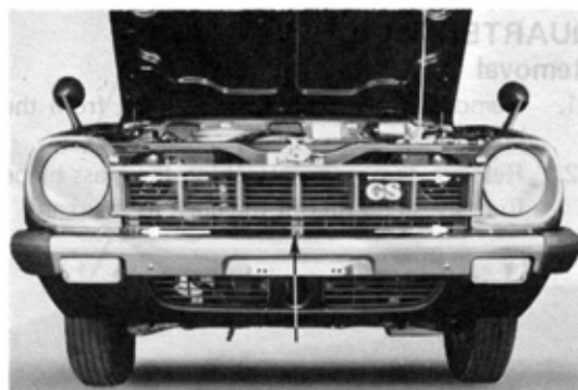
Fig. 2-143 Radiator Grille Removal
