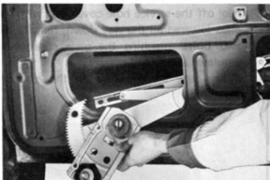
Fig. 2-29 Removing Window Regulator
