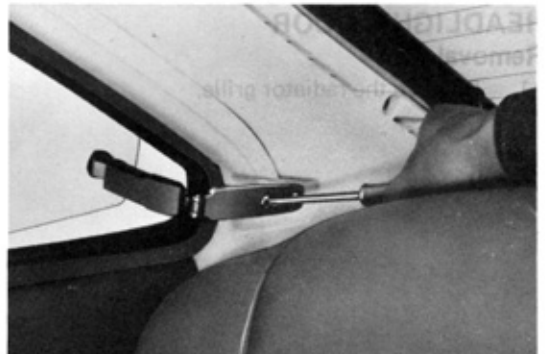
Fig. 2-146 Removing Quarter Window Lock
