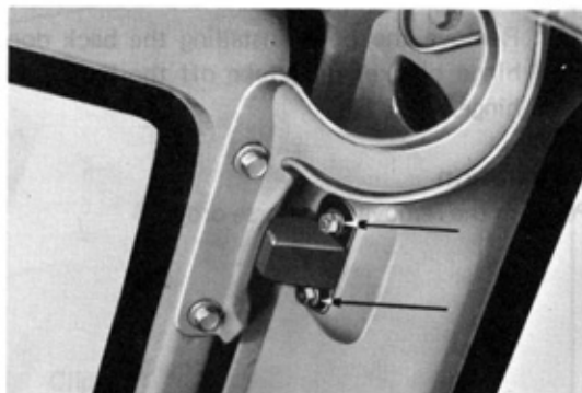
Fig. 2-159 Back Door Side Stopper Adjustment (2)
