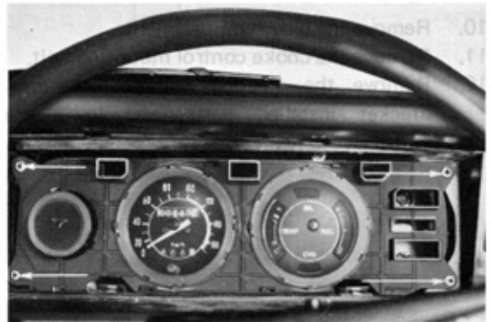
Fig. 2-74 Removing Combination Meter
