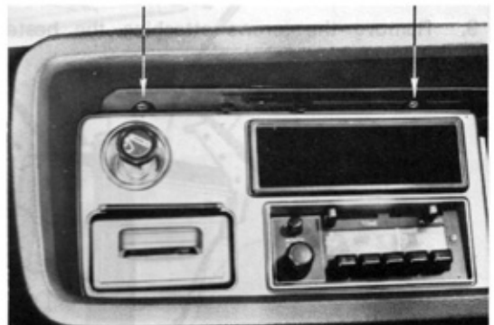
Fig. 2-73 Instrument Center Panel Removal
