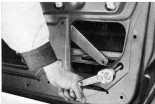
Fig. 2-25 Removing Door Glass
